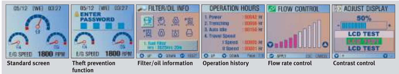
Control panel With color LCD display
